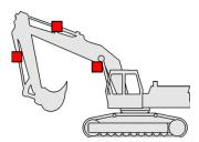
The load control valve is installed in the line to be protected between the main control valve and the hydraulic cylinder and is flanged directly on the cylinder. Additional pipework and piping between load control valve and cylinder is not permissible.
