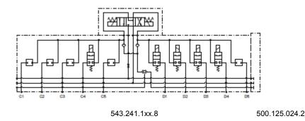
Example of a possible arrangement of different directional control valve sections.
