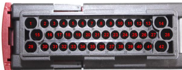
Pin-outs of the Plug-In Connector S1
