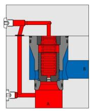
**Directional control valve function** with piloting source from port A.
