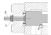
NOTE: A stroke limitation which is screwed in too far, will produce an unnecessary high loss.
